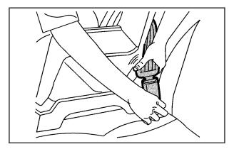
Push the latch plate into the buckle until it clicks. Make sure the release button is positioned so you would be able to unbuckle the safety belt quickly if necessary.
